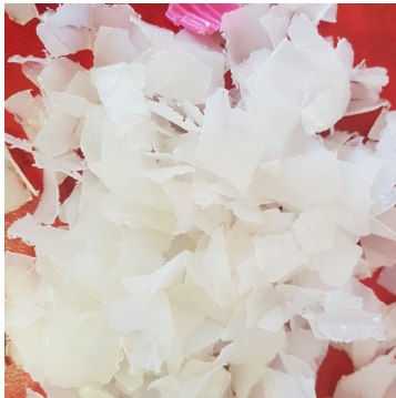
Figure 2: Perfectly clean HDPE flakes after applying the University of Sydney removal processes.
