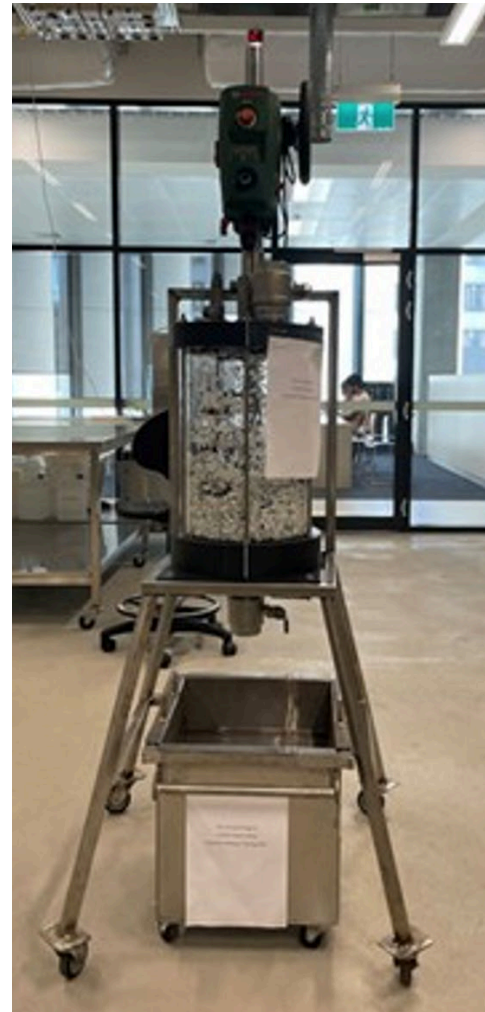
Figure 3.1: The test reactor. It represents about 2% of the throughput of the full scale plant.
